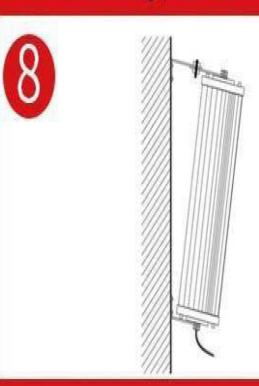
Screw the wall fixing plate to the top of the speaker. Fix the speaker in a position that needs to be fixed
