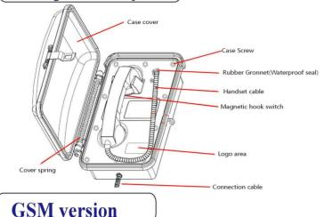
GSM 2G/3G Solar Powered with built-in rechargeable battery
