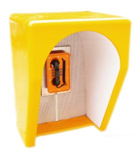
general-purpose resin material to BS476 Class 1 fire regulation, the RF-13 is extremely robust and weatherproof. Inside the hood's outer shell is a perforated polypropylene lining that houses 50mm non-hygroscopic acoustic insulation.
